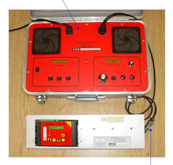
AC-PRO Direct Replacement Trip Unit Assembly Secondary Injection Test Connector
